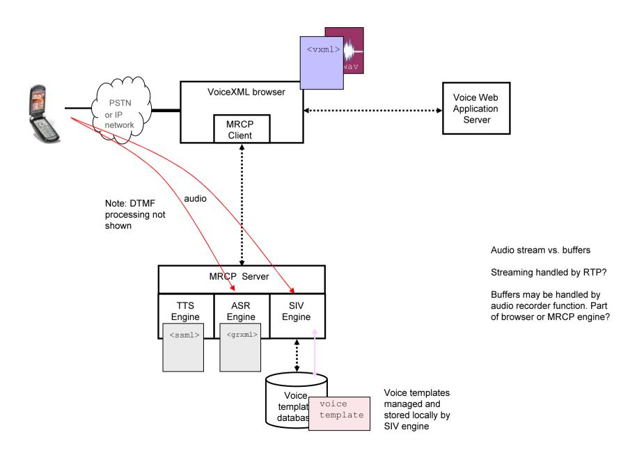
SIV engine managed by MRCP server SIV database managed by app server Voice model transmission managed by engine or MRCP Server
